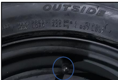
06.01 Cap for the inner tube of the wheel
