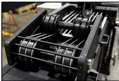
06.08 Pulley system for front CW cables
