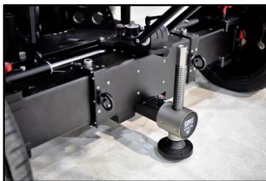
02.07 Dolly leveling jack introduced
