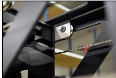
02.87 Rear top wheels second section
