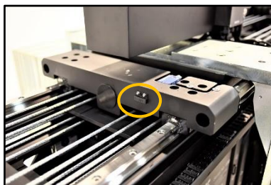
02.54 Magnet for extension limit
