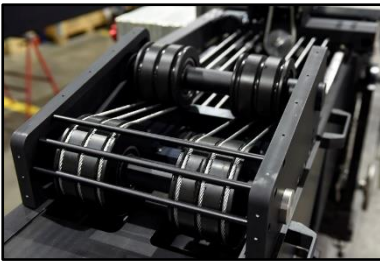
02.61 Pulley system for front CW cables.
