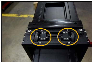
02.80 Top guiding wheels first section
