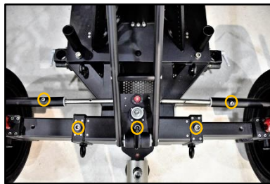
02.08 Screws to remove to collapse
