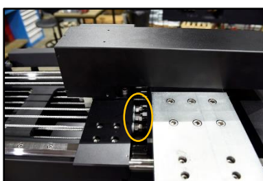
02.60 CW Cables ends in CW trolley
