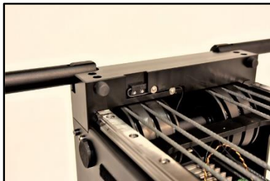
06.09 Pulley system for back CW cables
