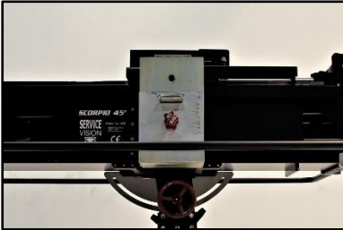
02.20 Counterweights in the center pos.
