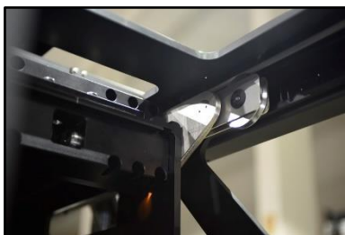
02.77 Rear top wheels in the first section
