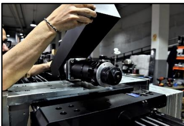
02.65 Motor for dynamic CW system
