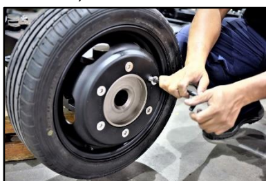
10.09 Assemble the wheels
