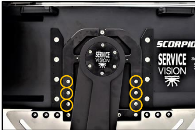
02.41 Left side screws for the arm
