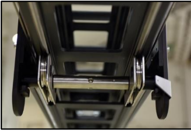
02.85 Front wheels in the first section
