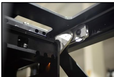
06.04 Rear top wheels in the first section
