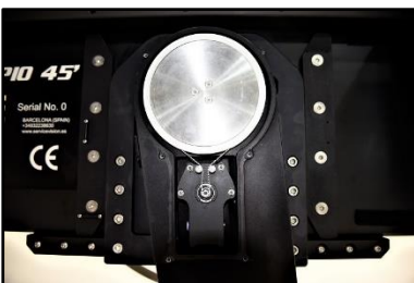
02.37 Tilt encoder (Ref. 7616) exposed
