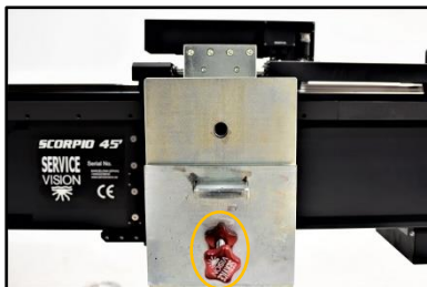
03.07 Telescopic Counterweights in the center
