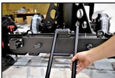
10.10 Assemble the steering handle
