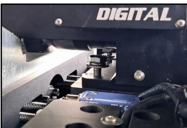
06.28 Rear screws from the CW motor block
