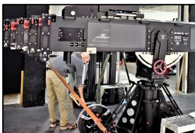
10.22 Front strap holding the arm
