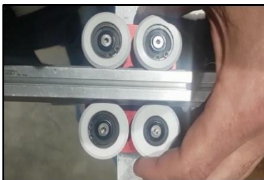
06.15 Adjusting the cable trolleys
