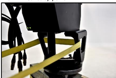
02.45 Leveling Head strap to front strap point.
