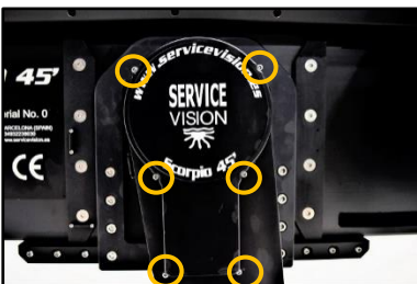
02.36 Tilt encoder cover and screws
