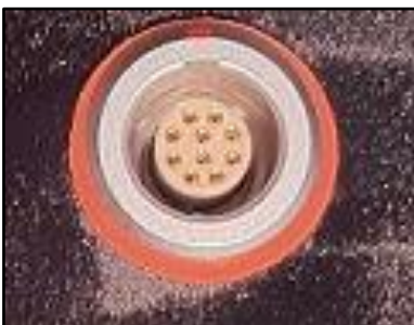
08.38 Encoder out from an EZ head
