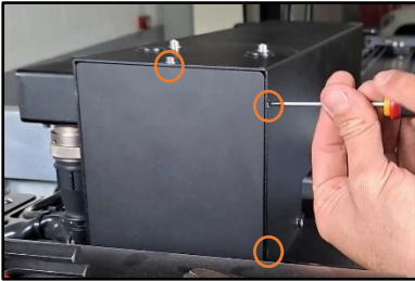
06.26 Screws from the front cover
