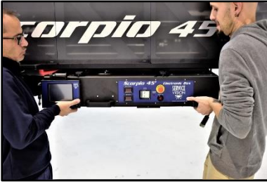
10.24 Sliding the electronic box
