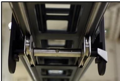
03.02 Guides of the telescopic sections
