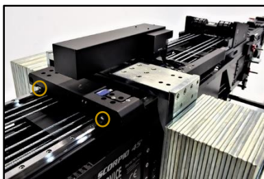
06.05 Bearing greasing points
