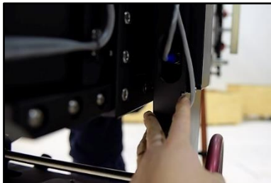
10.35 Connection of the tilt encoder
