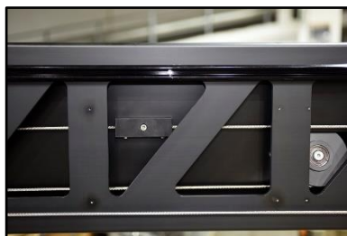
02.94 Rear pulley third section
