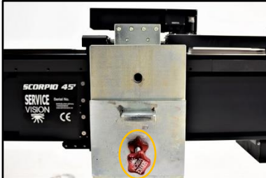
02.63 Telescopic Counterweights Screw and nut.
