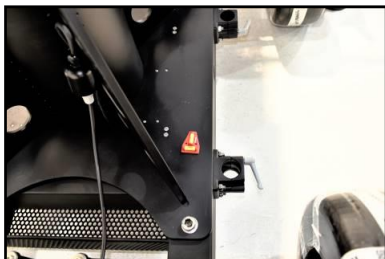
03.03 Bubble level on the base
