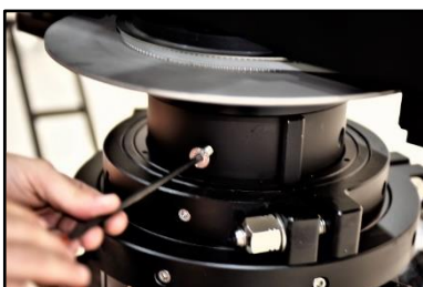
10.18 Tight the fulcrum to the column
