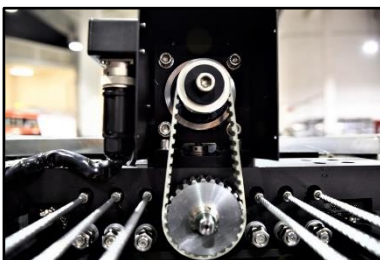
02.66 Belt and gear for the CW system
