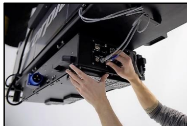
10.36 Connecting the EB side 1
