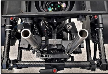
03.05 Camera not properly secured.
