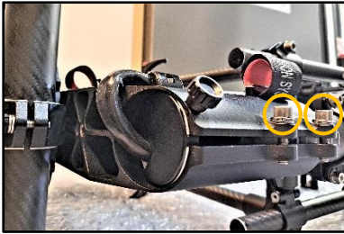
02.08 Bracers on side bars w/ screws marked
