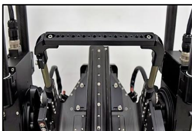
03.05 Upper bridge assembled.
