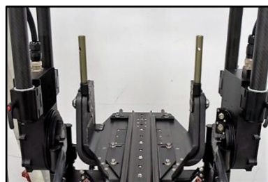
03.04 Bars assembled for upper bridge.
