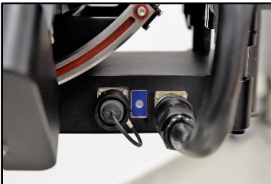
02.20 Right side connectors in the dog.
