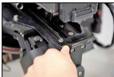
03.06 Safety pressed to slide the camera in.
