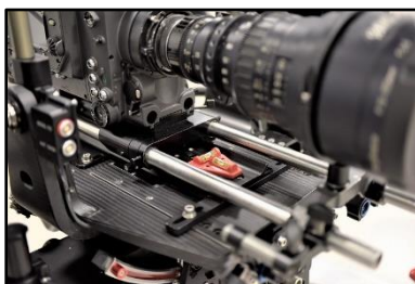
04.60 Position of the bubble level.
