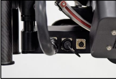
02.19 Left side connectors in the dog.
