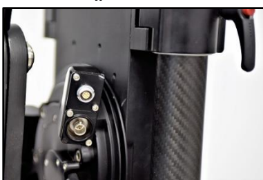
02.13 Connectors in master tilt.
