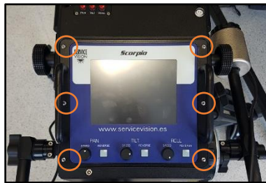
06.22 Philips screws from the frontal.
