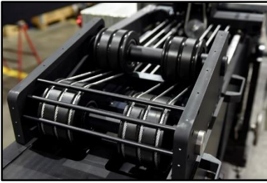
06.08 Pulley system for front CW cables
