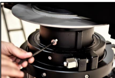
10.18 Tight the fulcrum to the column
