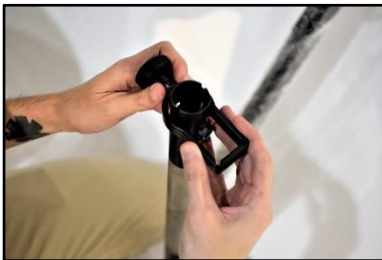
10.29 Slide the HC bracket before attaching the side bars
