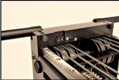
06.09 Pulley system for back CW cables
