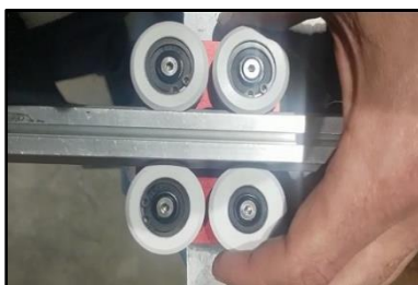
06.15 Adjusting the cable trolleys
