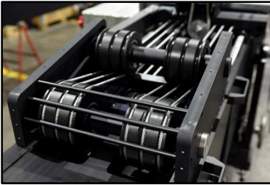
02.61 Pulley system for front CW cables.
