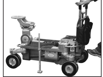
Easily lifts the PeeWee dolly for a tire change. Then, apply the brakes.
