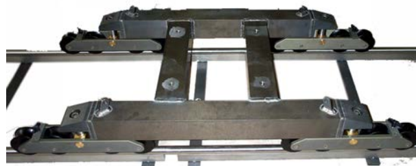
Mini base with Track wheel unit on GF-Track
