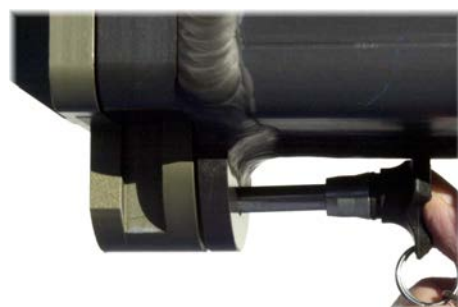
Securing the arm with a safety pin
