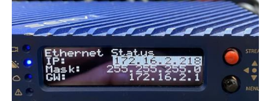
5, For succesful connection status should look similar to this and not be blank
