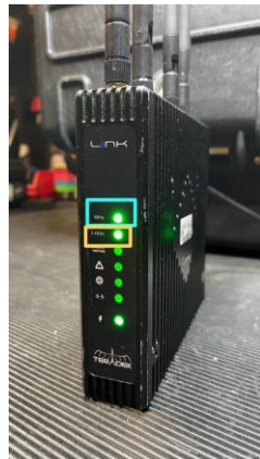
1, Turn on link and make sure these LED are lit up. Can take a few minutes
