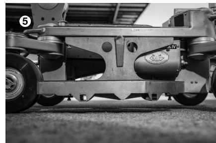
Adjust the two Thumb Screws on Side Board to take up play. #1645
