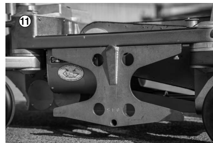
Adjust the two Thumb Screws on Star Plate to take up play. #1650
