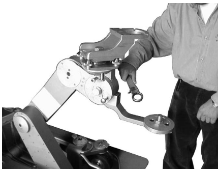
Tighten the Low Plate with the Universal Wrench #1689
